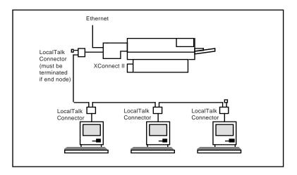
Figure 2-6 Connecting the XConnect II to a LocalTalk network
